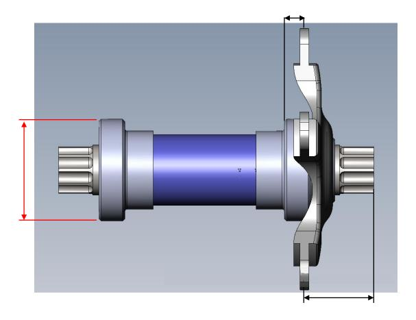
Bearing cup should fit to every bottom bracket shell!
