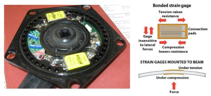
The handicap of Strain Gauges is the demand of temperature compensation and the effect of retardation.
