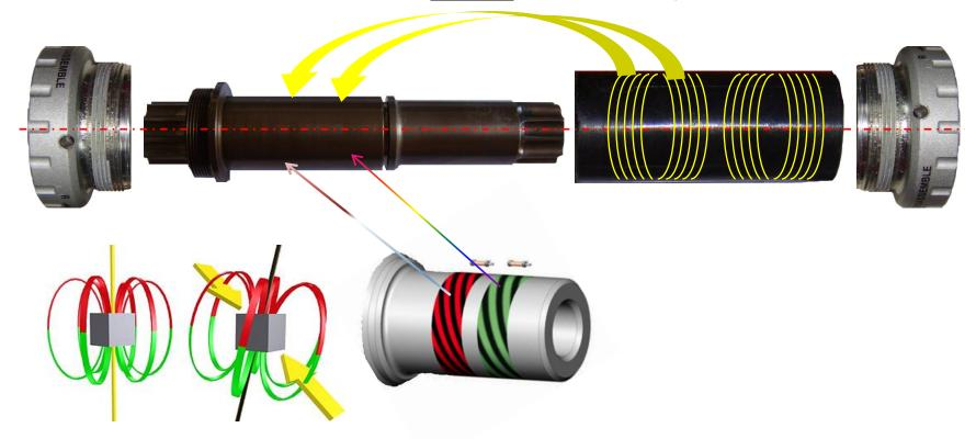
The Virelli effect says: Stress on a ferromagnetic body change its magnetic field.
