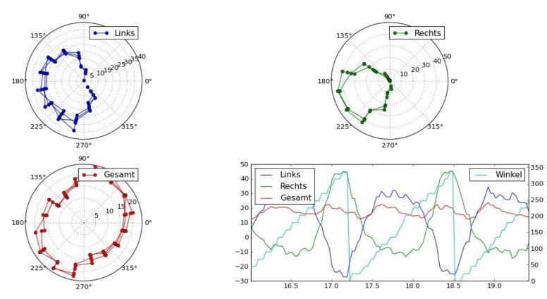
Time profile of torque development and compared to pedal angle
